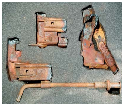
Fig.8 Typical items with a great number 'corrosion diodes'
